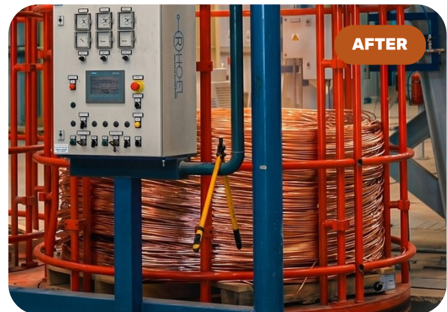
Rod and wire in standard diameters compliant with ASTM B49-98.
